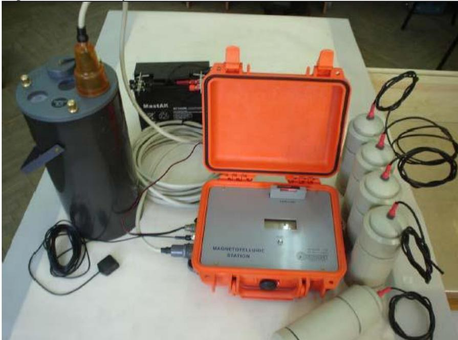
Fig. 1. Variant of MTS set with MF sensor on gimbal mechanic system of automatic stabilization of vertical position.
