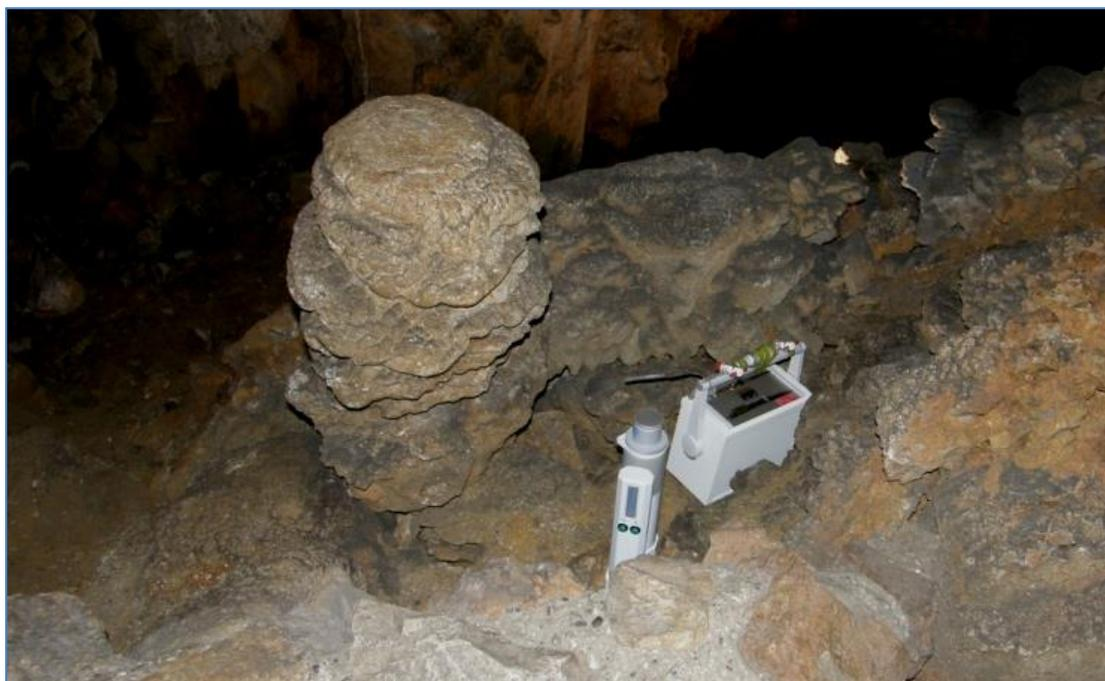
Figure 1 Combined measurements of radon using radon meter (right) and gamma spectrometer PRS-01(left) in the cave
